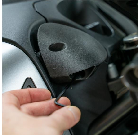
11. Ensure the bushings do not show signs of over tightening such as being excessively compressed or flaring out.
