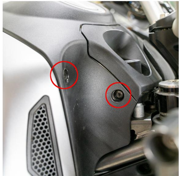
4. Begin by inserting the a 35mm mounting screw into the lower mounting hole of the deflector, then place the larger 8mm bushing on the mounting side for ease of installation.
