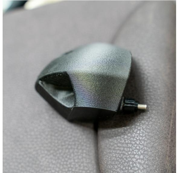
5. Hold the assembly, ensuring the bushing nor the screw fall out, and align it with the installation location.
