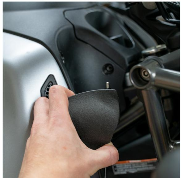
6. Fasten the screw with a 3mm Allen tool. Tighten loosely to allow ease of rotation, final tightening occurs later.
