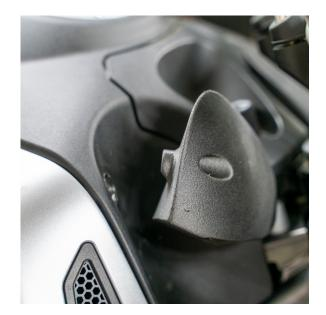
8. Insert the a 35mm mounting screw into the upper mounting hole of the deflector. Now using the smaller 4mm bushing, hold the 4mm bushing on the mounting side for ease of installation.
