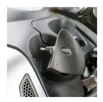
9. Tilt the deflector, with the mounting screw and bushing, towards the back of the bike for installation. Using the 3mm Allen tool, thread the mounting screw in and tighten to final tightness (♠hand tighten only, do NOT overtighten)
