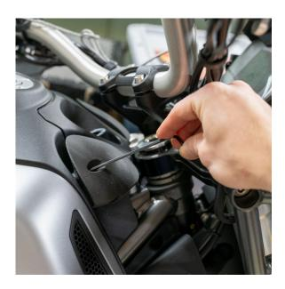
10. Return to the lower mounting screw and, using the 3mm Allen tool, tighten to final tightness (♠ hand tighten only, do NOT overtighten)
